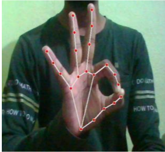
Fig 5.6: Gesture for scroll down function
