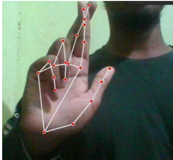
Fig 5.10: Gesture for typing or clicking a letter on screen from virtual keyboard
